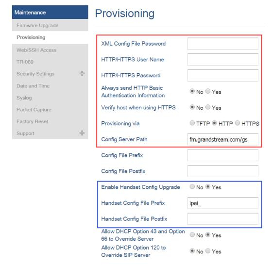
**Provisioning via**: Choose the method that the base station uses to request handset ipei config file. Can use TFTP, HTTP or HTTPS.
