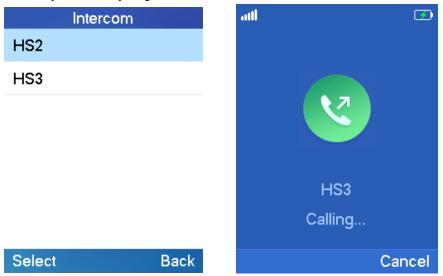
If the Intercom call failed, please check if the handset has a valid SIP account registered and Direct IP call is enabled.
