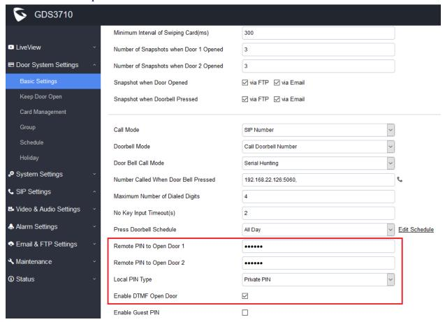
For remote PIN to open door, the PIN can be configured in above setting.
