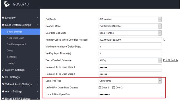
If Unified PIN (Universal PIN) is configured to open door, then which door can be controlled by the PIN is configured in the UI once "Unified PIN" selected.
