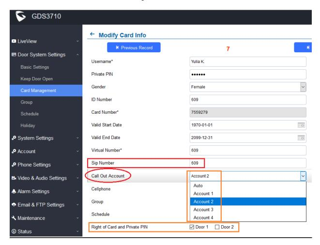
For special situation where no RFID card is assigned, system administrators can manually create a fake non-duplicable random number as "Card Number" (this is the database index, cannot be empty) but associate it with created PIN or SIP number or Virtual Number, as well as the Schedule or Group to control the door access privilege. Like for example, create these for guests, temporary or seasonal employees, cleaning ladies, contractors or UPS/FedEx person or postman.
