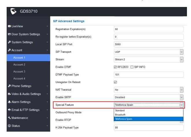
In the device web UI  $\rightarrow$  Account X (X=1, 2, 3, and 4)  $\rightarrow$  SIP Advanced Settings  $\rightarrow$  Special Feature: There is a new feature specially designed for Telefonica Spain to match the service provided by Telefonica to their customers. Just need to enable this feature via either WebUI or Provisioning.
