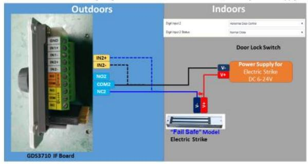
GDS3710 Connection & Wiring Diagrams ---- "Fail Safe" Electric Strike, 3rd Party Power Supply
