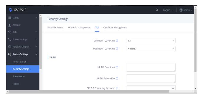
Allow the GSC3505/GSC3510 to accepting the connection from the lower TLS version.
