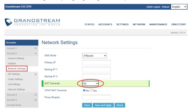
The IP phone or GSC3570 can use any empty account, meaning while default Account 1 registered to UCM/Proxy, the blank Account2 can be used to IP call. (but need to select this account to be "Active").
