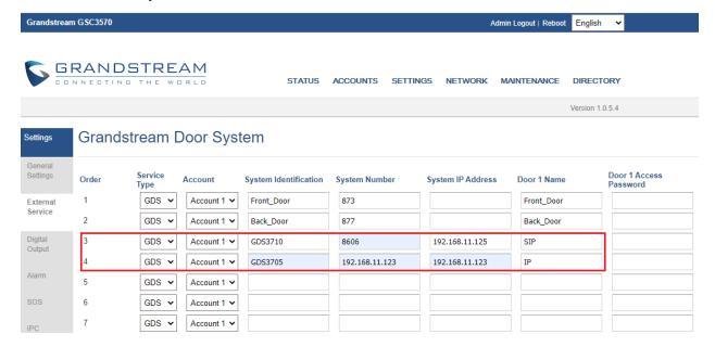
There is no door limitation for such usage but only ONE DOOR can be opened at one time. It is just a typical SIP call open door application.
