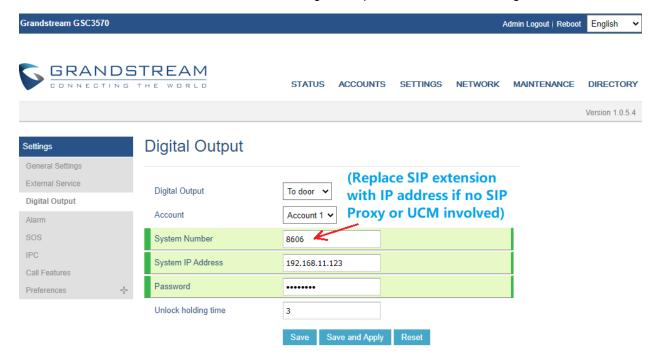
Also if the solution or system integration is using static IP address without SIP Proxy, all the devices involved (GDS/GSC/IP Phone) should choose "NAT Traversal" to "No" and should NOT "Use Random Port", otherwise it will cause ghost call (SIP signaling working but NO media).
