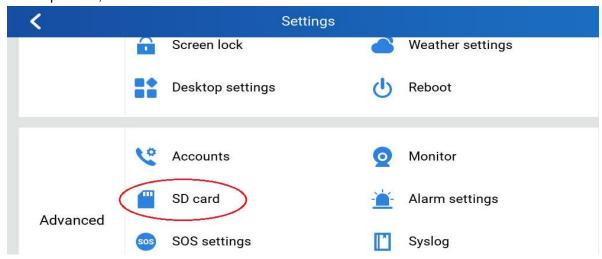
Thouch the "Format" to perform SD card initialation and mount. All the SD card has to be formatted by GSC3570 before usage.
