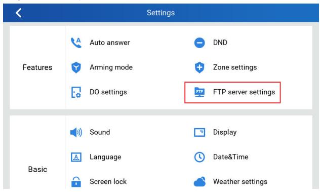
By default the FTP Server is disabled. Touch to "Enable" the FTP, the configure the Port used, create username and Password.
