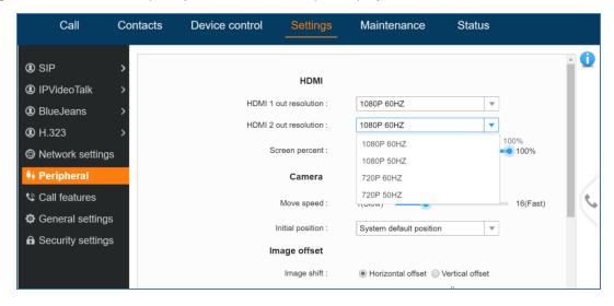
The P value for this option is P25105. 10 - 1080P 60HZ, 9 - 1080P 50HZ, 6 - 720P 60HZ, 5 - 720P 50HZ. Default value is 10.
