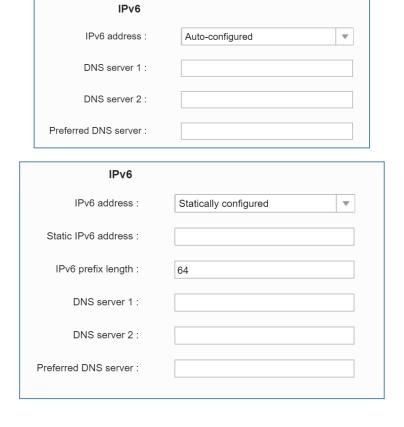
When IPv6 is used on GVC320x, the following format needs to be used:
