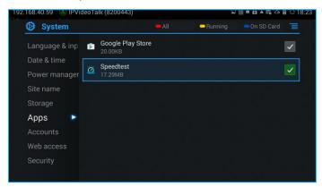
Choose the target app that needs to be moved to SD card to see detailed information. Then Click on "Move to SD card" to make the change take effect. After configuration, the app will not be listed on GVC320X device after the external SD card is ejected.
