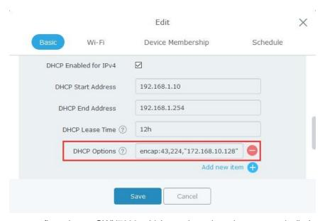
For DHCP server configuration on GWN7000, which translates the values automatically, is as follows:
