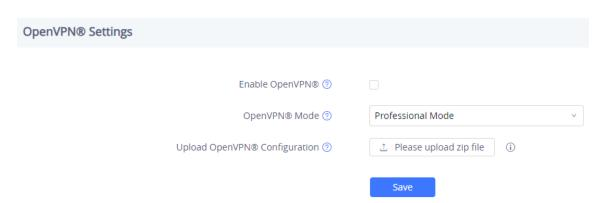
This feature allows the user to choose whether to use "Simple Mode" or "Professional Mode" for OpenVPN configuration. The "Simple Mode" provides a basic set of parameters on the web UI for OpenVPN. The "Professional Mode" allows the user to upload an OpenVPN configuration for a more customized setup for VPN. Note: Please see OpenVPN configuration upload guide on the Grandstream product page for additional details.
