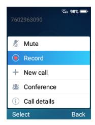
If enabled the device can record audio during a call. If disabled, this feature is hidden during a call.
