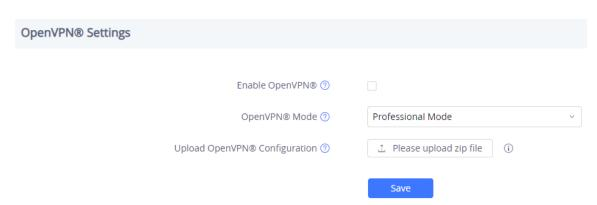
This feature allows the user to choose whether to use "Simple Mode" or "Professional Mode" for OpenVPN configuration. The "Simple Mode" provides a basic set of parameters on the web UI for OpenVPN. The "Professional Mode" allows the user to upload an OpenVPN configuration for a more customized setup for VPN. Note: Please see OpenVPN configuration upload guide on the Grandstream product page for additional details.
