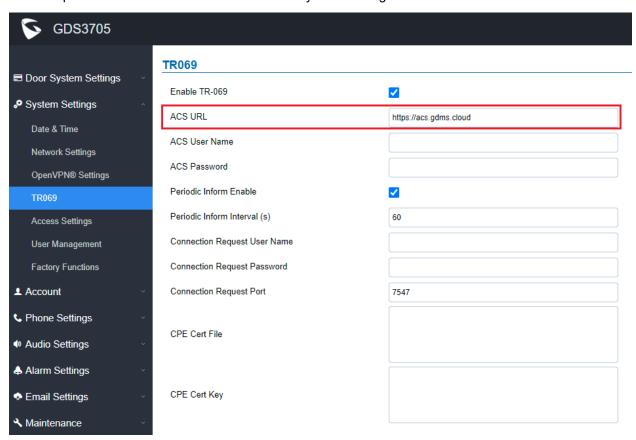
If service providers support TR069 provisioning, or users have account of GDMS service, the GDS3705 can be configured via using related configuration template in the TR069 server or GDMS server side, then provisioning it over the Internet (Cloud Service).
