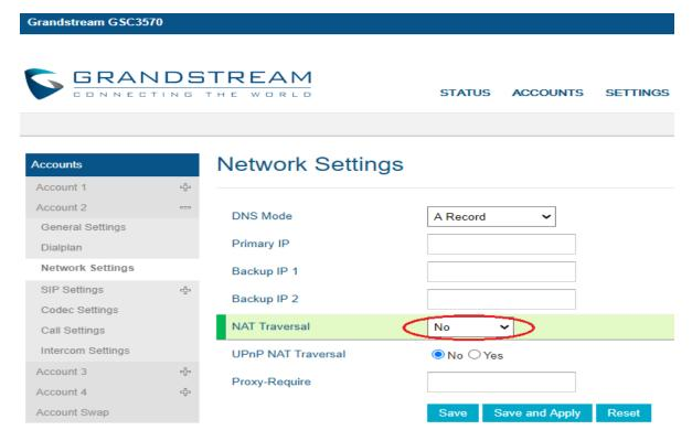
The IP phone or GSC3570 can use any empty SIP account, meaning it can be mixed if Account 1 registered to UCM/Proxy and Account 2 (blank) to use IP (but the account has to be configured as "Active").
