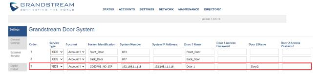
In the "SETTINGS → External Service", input the IP address of GDS37xx where the GSC3570 paired with, and input the correct PIN for open related remote doors. The PIN should match with GDS37xx related remote PIN to open door.
