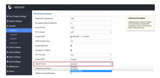
In the device web UI  $\rightarrow$  Account X (X=1, 2, 3, and 4)  $\rightarrow$  SIP Advanced Settings  $\rightarrow$  Special Feature: There is a new feature specially designed for Telefonica Spain to match the service provided by Telefonica to their customers. Just need to enable this feature via either WebUI or Provisioning.
