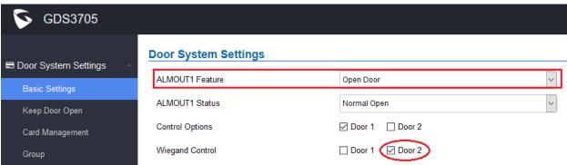
If ALMOUT1 (COM1) interface is set to control DOOR2 opening, "Lock Status" can be configured by choose "Normal Open" or "Normal Close" based on the strike used.
