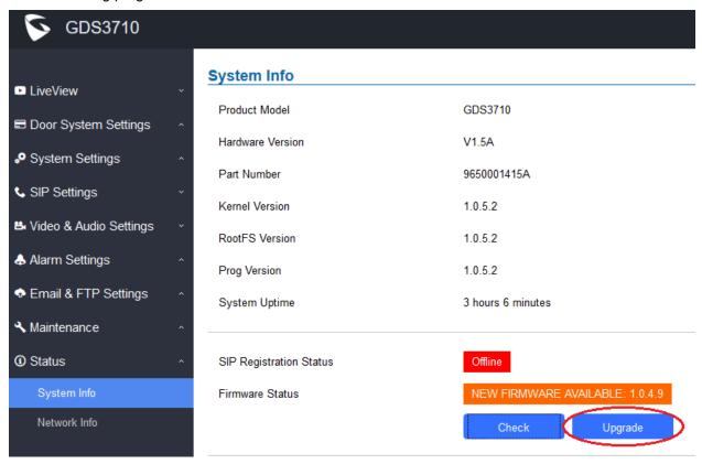
Please do NOT power off the device when firmware burning/upgrade is in processing.
