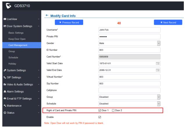
If using RFID card or Private PIN to open door, then which door can be opened by the RFID card or Private PIN is configured via "Card Management", see above screenshot.
