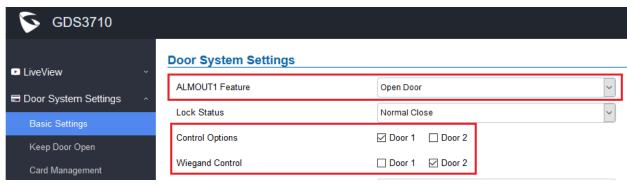
If Alarm\_Out (COM1) interface is set to control Door2 opening, "Lock Status" can be configured by choose "Normal Open" or "Normal Close" based on the strike used.
