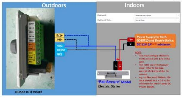
GDS3710 Connection & Wiring Diagrams ---- "Fail Secure" Electric Strike, 3rd Party Power Supply
