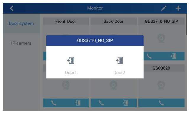
Press related "Door 1" or "Door 2" icon (two doors configured in this example), the GDS37xx will operate the strike and open the correspondent door accordingly.
