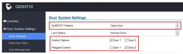
If Alarm\_Out (COM1) interface is set to control Door2 opening, "Lock Status" can be configured by choose "Normal Open" or "Normal Close" based on the strike used.
