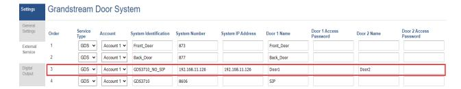
In the "SETTINGS → External Service", input the IP address of GDS37xx where the GSC3570 paired with, and input the correct PIN for open related remote doors. The PIN should match with GDS37xx related remote PIN to open door.
