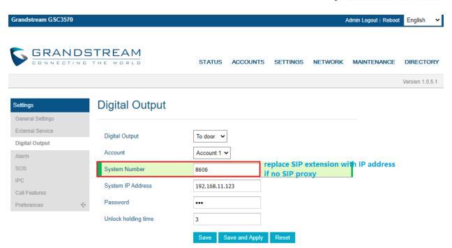
If the solution/integration is using static IP address without SIP Proxy, all the devices involved (GDS/GSC/IP Phone) should choose "NAT Traversal" to "No" and should NOT "Use Random Port", otherwise will have problem of ghost call (SIP signaling working but NO media).
