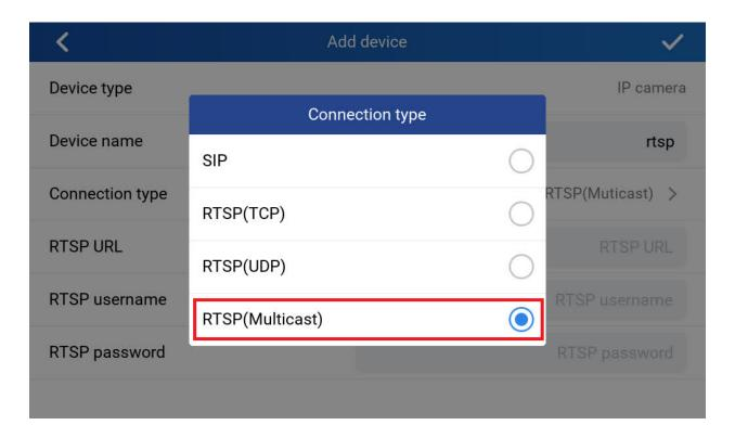
Touch to choose "RTSP (Multicast)" if the IP camera will be configured using Multicast mode.
