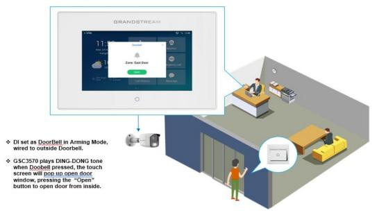
The wiring example of GSC3570 as doorbell and open door:
