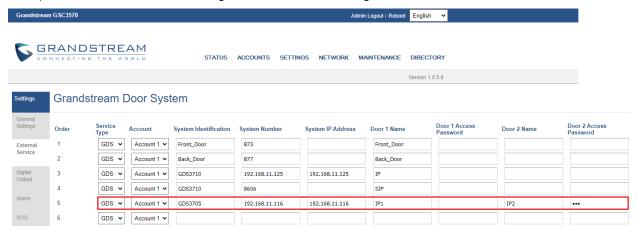
Also, the web UI configuration in "Maintenance  $\rightarrow$  LCD Access  $\rightarrow$  Door settings":
