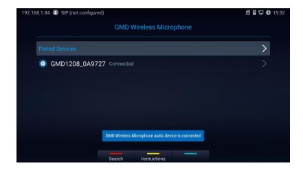
After entering the GMD Wireless Microphone menu, the GMD1208 in wireless mode can automatically pair with GVC3220 when connected via USB.
