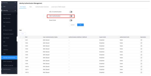
MAC authentication has been added to the port authentication method, and the authentication methods support RADIUS and Local.
