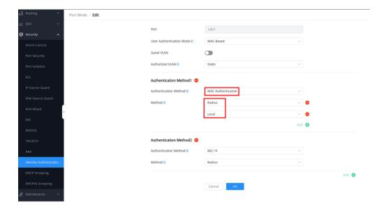
To add a MAC-based local user, you need to add the MAC address, port control mode, VLAN authorized for use after authentication, re-authentication time, and inactive time.
