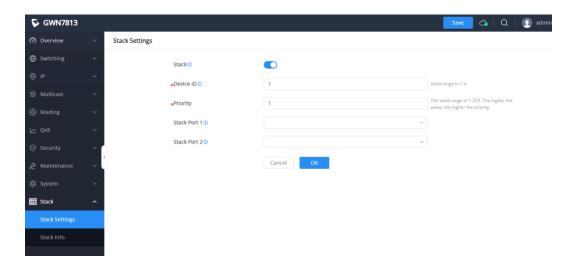
Note: After the configuration is completed through the CLI or Web GUI, you need to save it first, then restart the device. The device ID and port number will take effect after the restart is completed.
