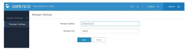
When device boot in factory default, by login in Slave mode, you can add the IP address of your GWN
